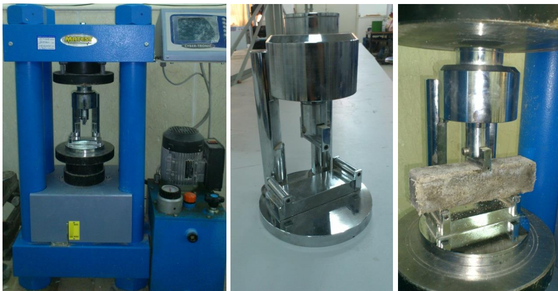
Figure 3: Flexural strength test machine and specimen inside the testing machine
