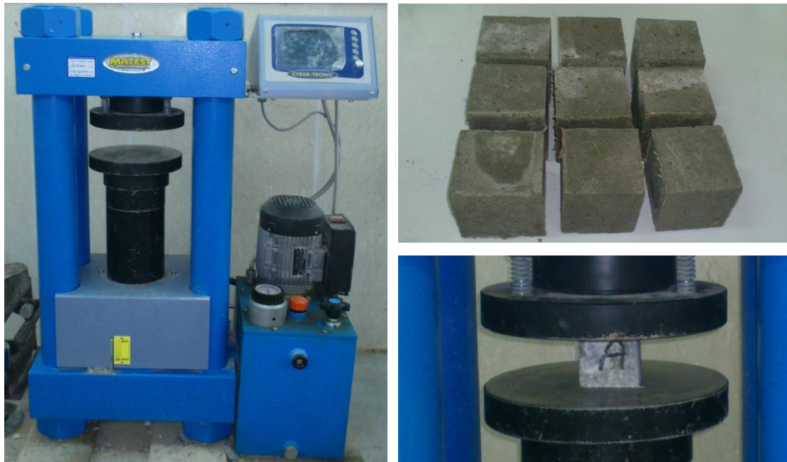
Figure 2: a) Compressive strength test machine. b) Test specimens 50 \times 50 \times 50 \text{ mm}^3 cubes. c) Specimen inside the testing machine.
